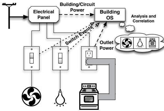
Fig. 1. Our monitoring and control architecture.
