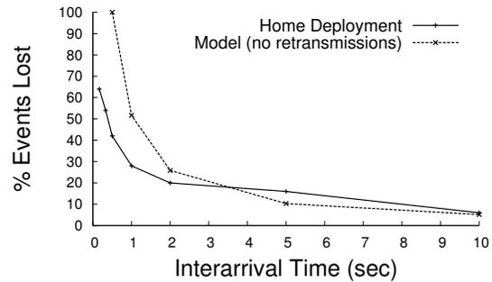
Fig. 3. Switch events may collide with outlet queries.
