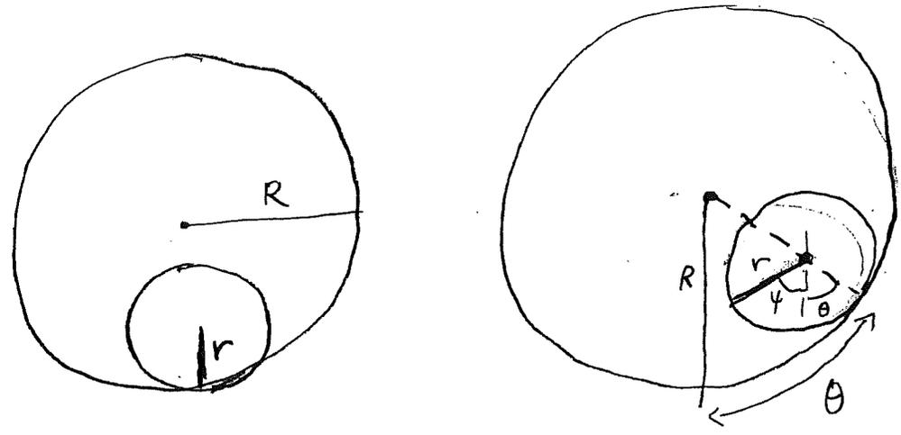
$\psi =$  angle inner pipe has turned w.r.t. vertical.
