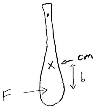
A force  $F$  is applied for a short time interval  $\Delta t$  at a distance  $b$  below the cm. of some object.
