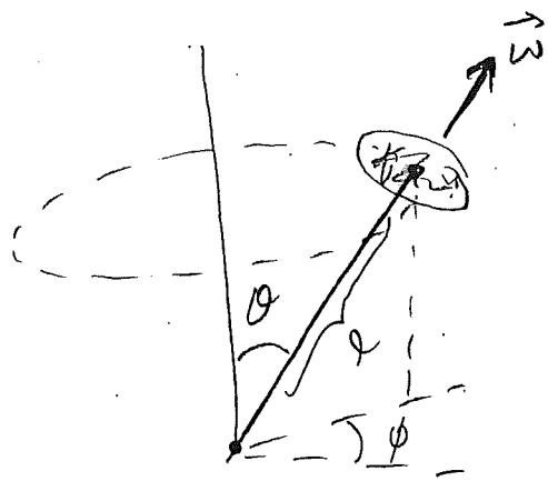
The external gravitational torque will cause it to precess around a vertical line w/ precession frequency  $\dot{\phi}$  given approximately by  $\frac{mgl}{I\omega}$
