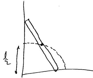
Note that when the ladder hits the ground, the horizontal velocity ( $\dot{x}$  = moment) is zero.
