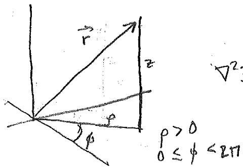
$$\nabla^2 \Phi = \frac{1}{\rho} \frac{\partial}{\partial \rho} \left( \rho \frac{\partial \Phi}{\partial \rho} \right) + \frac{1}{\rho^2} \frac{\partial^2 \Phi}{\partial \phi^2} + \frac{\partial^2 \Phi}{\partial z^2} = 0$$
