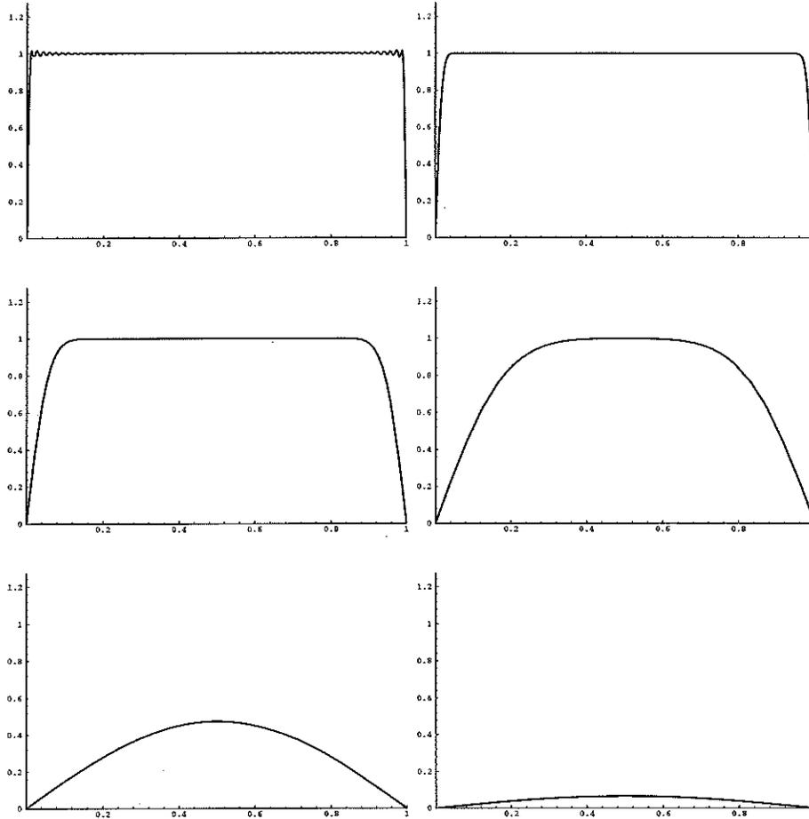
Figure 2: Thermal time evolution of square wave (with 60 terms) at  $t = 10^{-5}$ ,  $10^{-4}$ ,  $10^{-3}$ ,  $10^{-2}$ ,  $10^{-1}$ , and 0.3
