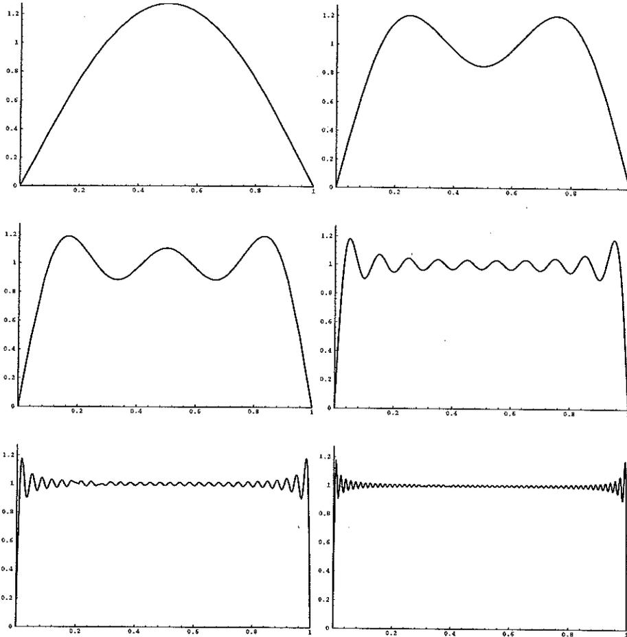
Figure 1: Fourier decomposition of square wave with 1, 2, 3, 10, 30, and 60 terms
