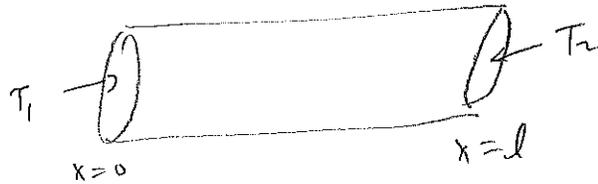
$$T(x) = T_1 + (T_2 - T_1) \frac{x}{l}$$
