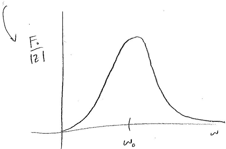
Power dissipated by a damped driven oscillator (Steady state)
