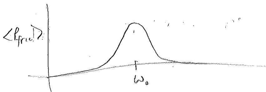
$$\text{max power dissipated at } \omega = \omega_0, \text{ where } (2) = b$$
