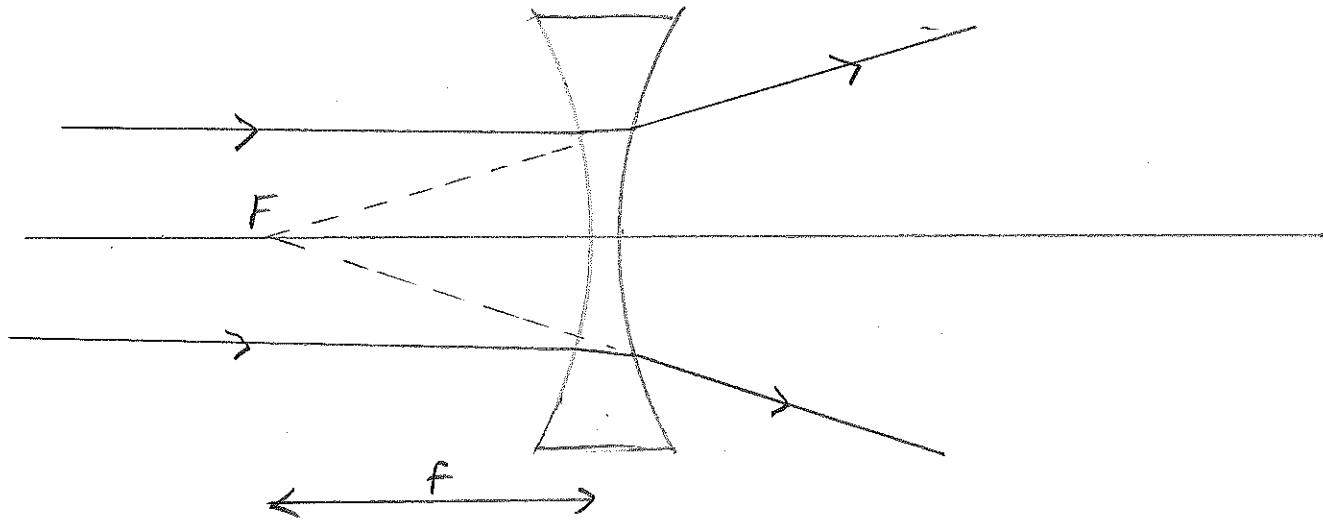
For a diverging lens,  $F$  is a virtual focus because rays appear to come from it, but do not actually pass through it
