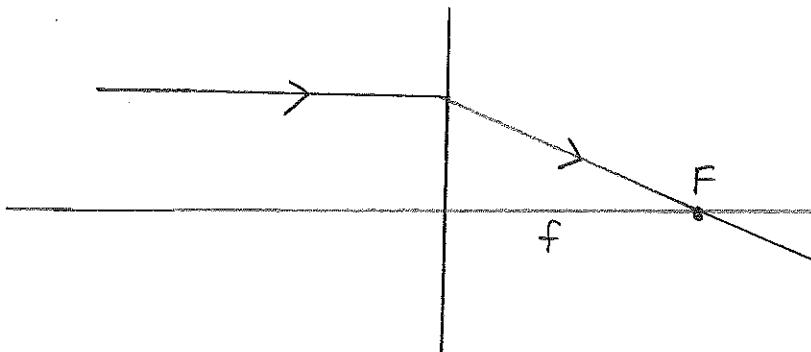
① a paraxial ray is refracted through  $F$
