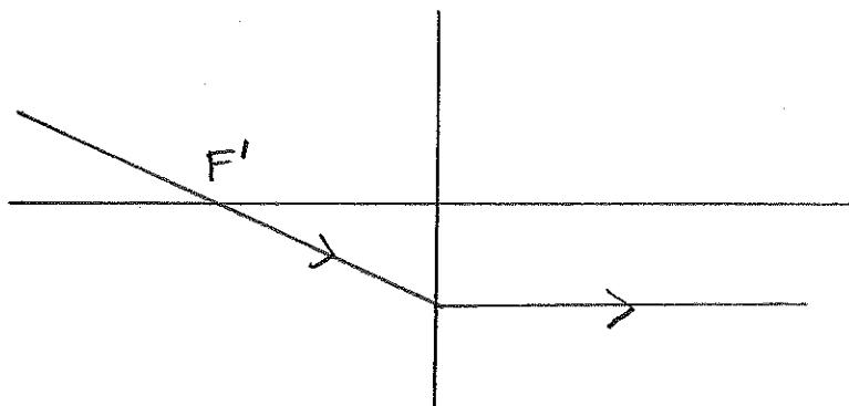
② a ray passing through  $F'$  is refracted parallel to axis
