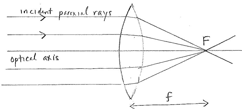
Paraxial rays (= rays parallel and close to the optical axis)
