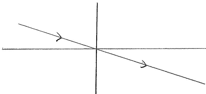
③ a ray passing through the center of the lens is undeviated (parallel surfaces)
