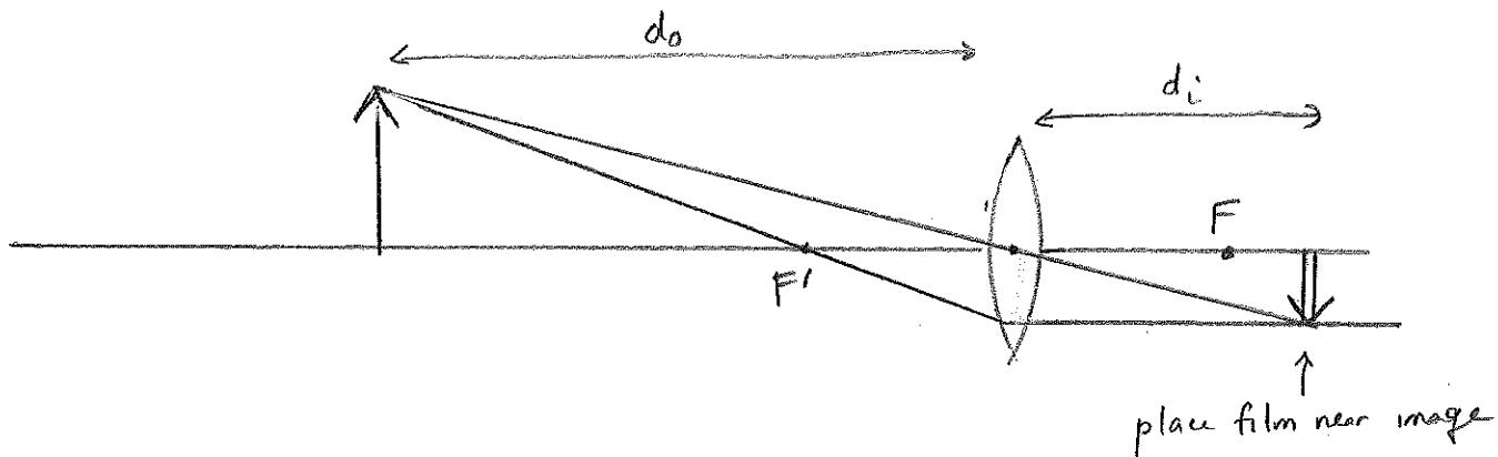
"Focusing a camera": adjusting  $d_i$  (distance from lens to film)
