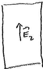
$\vec{E}_2$  = electric field of (polarized) light emerging from second filter
