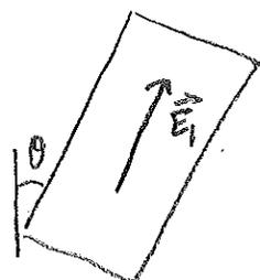
$\vec{E}_1$  = electric field of (polarized) light emerging from first filter (light coming toward you)
