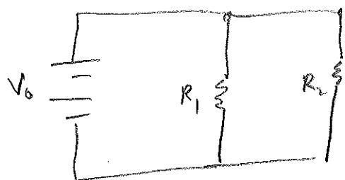
Voltage drop across each resistor connected in parallel is the same
