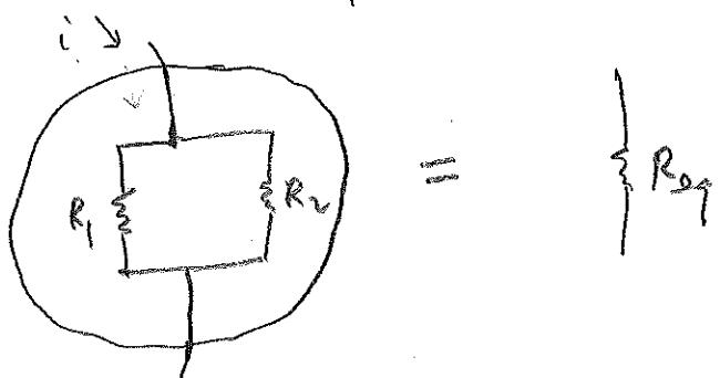
Two resistors connected in parallel are equivalent to a single resistor  $R_{\text{eq}}$  where
