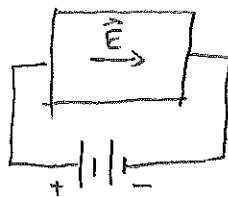
In a conductor, an electric field  $\vec{E}$  acting on conduction electrons results in constant drift velocity
