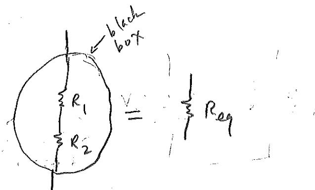
Two resistors connected in series are equivalent to a single resistor of resistance.
