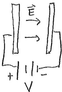
In vacuum, an electric field  $\vec{E}$  acting on an electron results in acceleration
