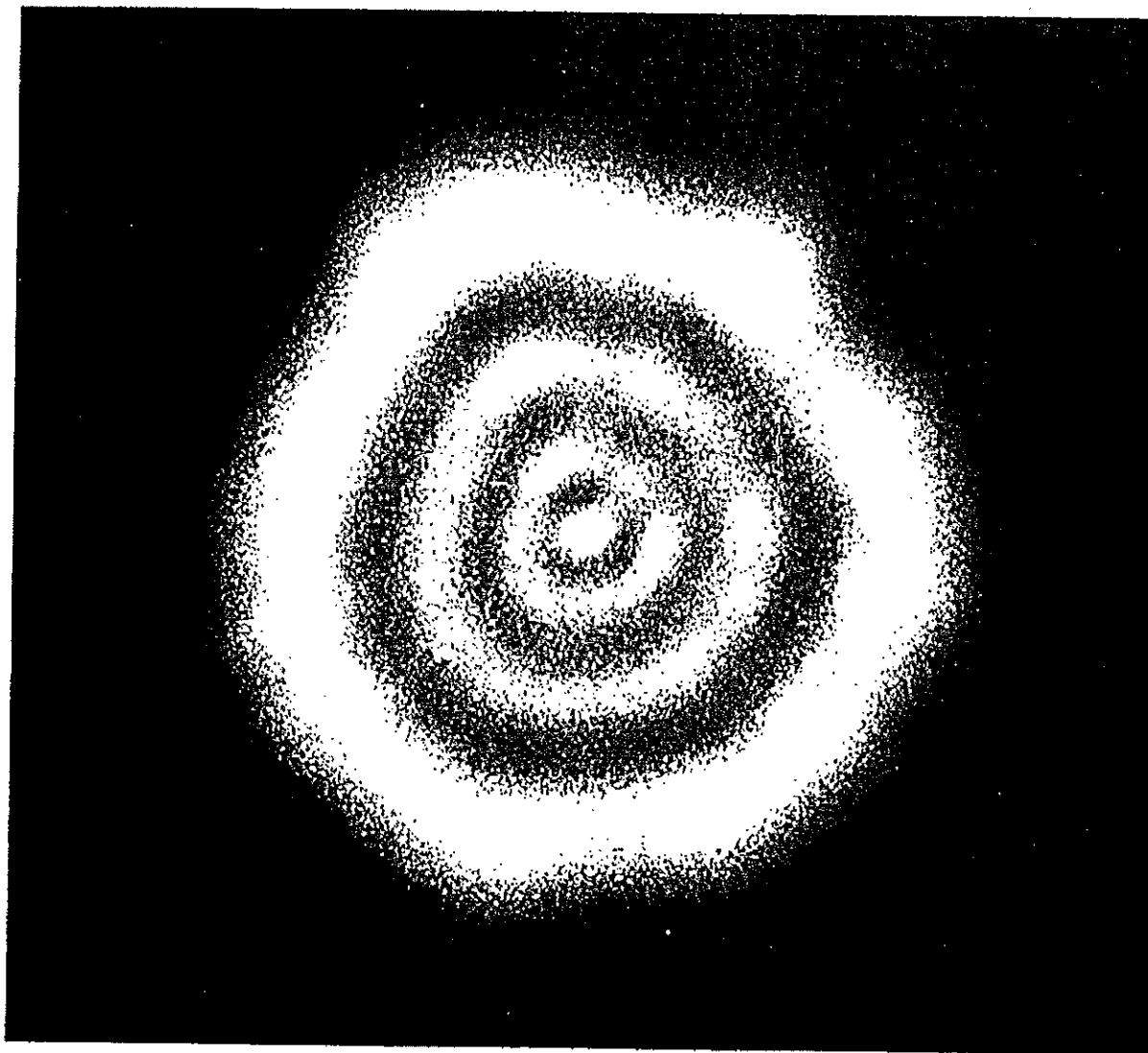
Figure 2 An electron diffraction pattern using a circular aperture of diameter 30\ \mu\text{m} and 100-keV electrons. Compare with the optical pattern (Fig. 2 of Chapter 46).
