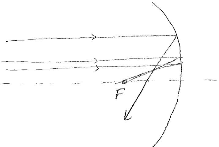
Fact that not all rays reflect to F is called spherical aberration.
