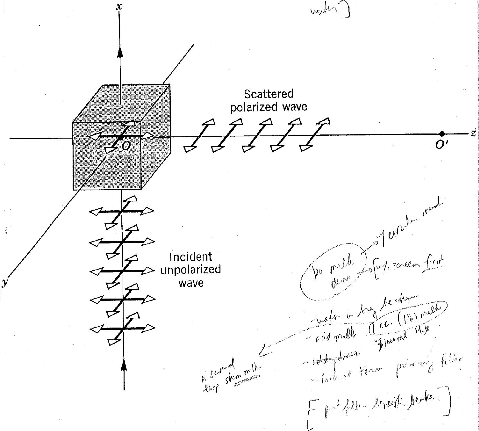
Unpolarized light, when scattered thru 90°, will be completely polarized.
