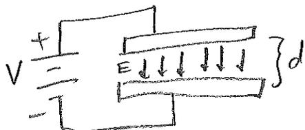
If the plates are close together, the battery creates an approximately uniform electric field  $E$  between the plates
