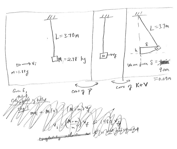
$\Delta K + \Delta V = 0$   $(0 - \frac{1}{2}(m - m)v_f^2) + (m + m)gh - 0 = 0$   $V_f = \sqrt{2gh}$   $h = L - \sqrt{12-8^2} = 0.00109 m$   $v_f = 0.146 \%$   $V_k = \frac{m + m}{m}v_f = 1480v_f = 217 \%$
