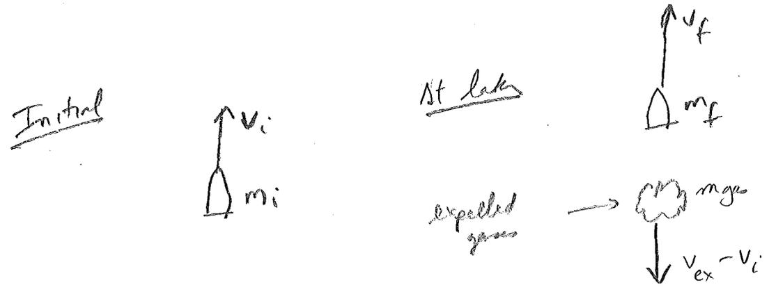
gases are expelled from rocket w/ relative velocity  $v_{ex}$
