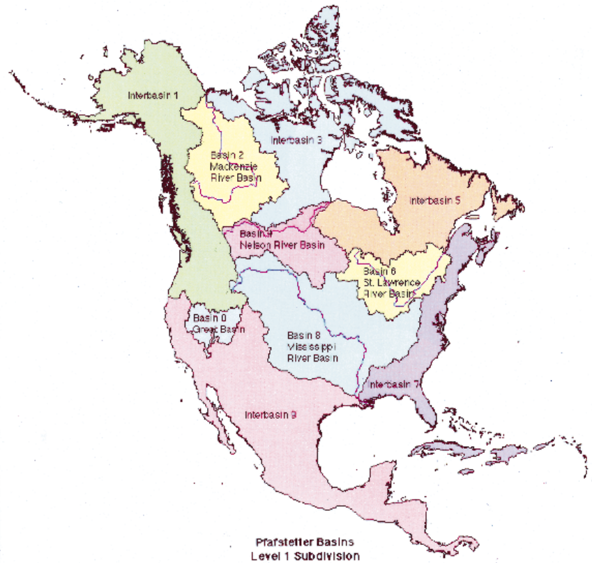
Fig. 2. Subdivision of the North American continent into Pfafstetter basins using the GTOPO30 DEM from USGS.
