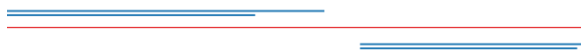
Figure 3. Line segments from Hough transform (blue) are merged to one or more collinear line segments (red).
