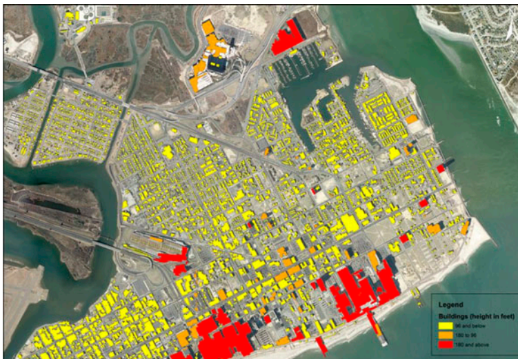
Figure 8. Map showing building heights in different categories derived from LiDAR point clouds.
