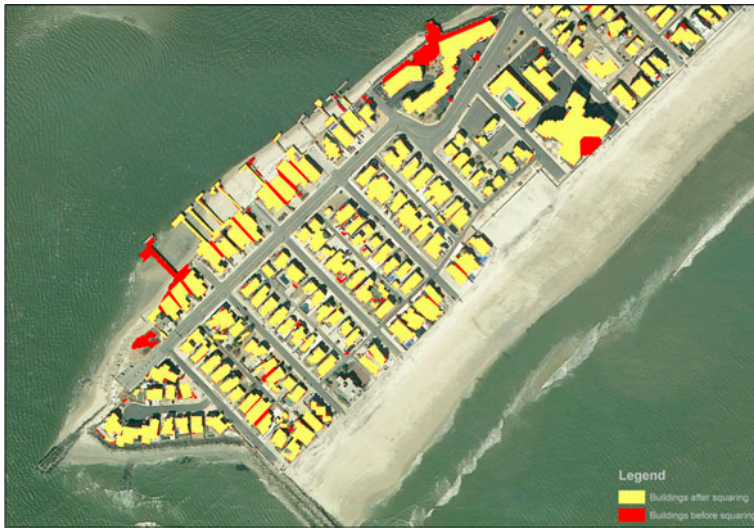
Figure 4. A sample data-set from Longport Borough showing buildings before and after applying squaring function.
