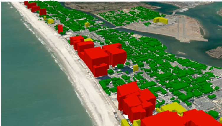
Figure 10. 3D depiction of the building structures derived from LiDAR data in ArcScene 10.1. Buildings are shown as high-rise (red – 180 ft and above), mid-rise (yellow – 180–96 ft) and low-rise (green – 96 ft and below).
