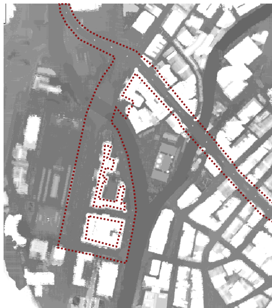
Fig. 13. Fusion of top-view LiDAR and ground-view SfM point-cloud data; the dotted line refers to the ground-view SfM data boundary.
