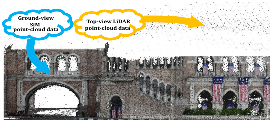
Fig. 12. Example of a point-cloud data fusion obtained by blending the top-view LiDAR data with the ground-view SfM data.
