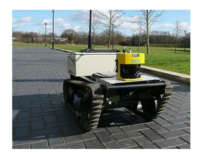
Robot equipped with LiDAR: uses it to construct maps and avoid obstacles
