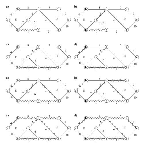
To implement Kruskal's idea, we need to a structure that maintains the "partial" trees and is able to support the following operations: (a) initialize a tree as consisting of a single vertex; (b) are two vertices in the same tree?; and (c) join two trees together.
