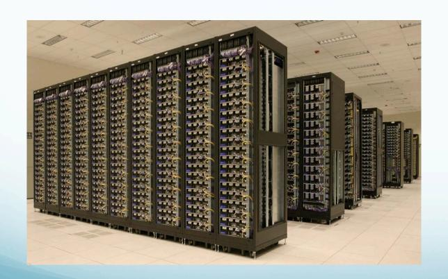
Bowdoin computing grid: 16, 32 and 40 core machines, 128GB RAM >500 cores!
