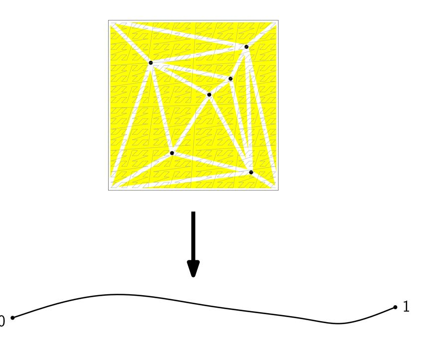
Quadtree cell  $\equiv$  interval on Z-order curve
