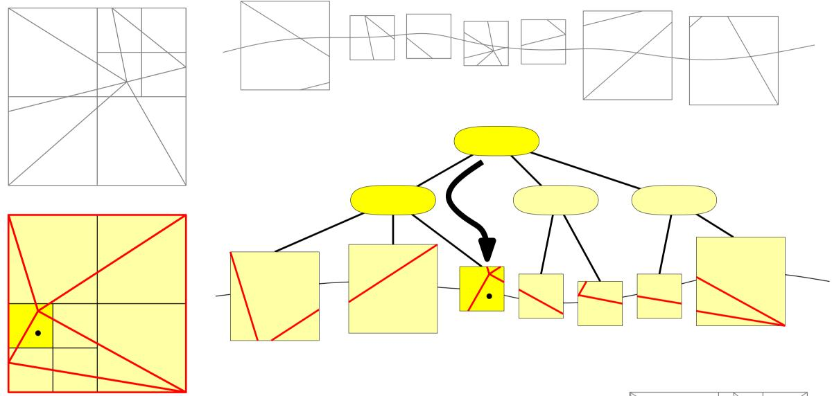
n: number of triangles; B: disk block size Ideally: O(n) quadtree cells, O(1) edges each
