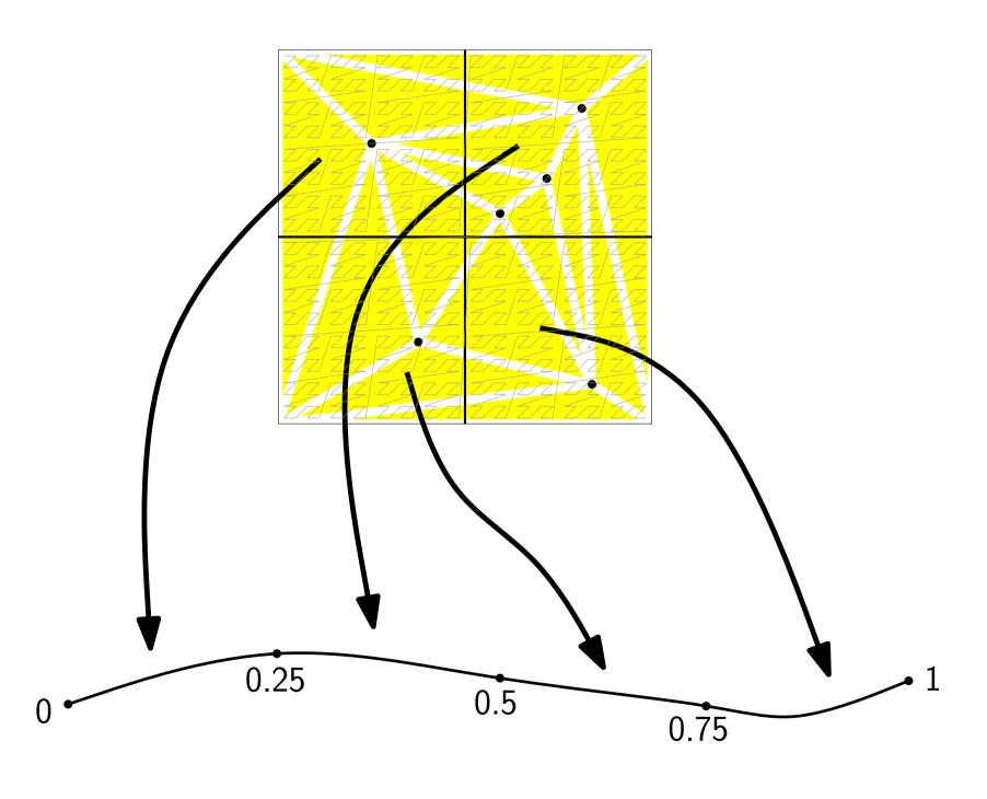
Quadtree cell  $\equiv$  interval on Z-order curve
