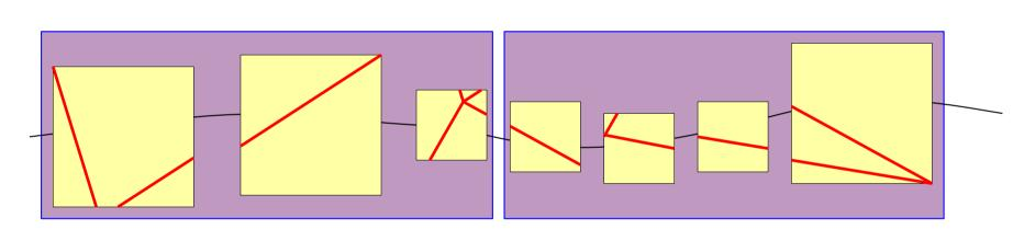
n: number of triangles; B: disk block size Ideally: O(n) quadtree cells, O(1) edges each
