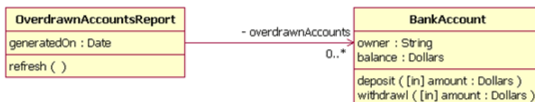
Figure 7: An example of a uni-directional association: The OverdrawnAccountsReport class knows about the BankAccount class, but the BankAccount class does not know about the association.
